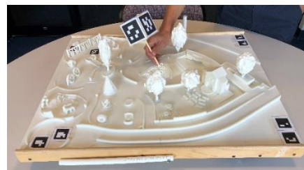
Fig. 1. 3D printed version of playground map, shown with user holding pointing stylus.
