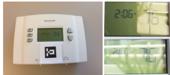
Figure 1. (a) Appliance with LCD display, with marker affixed below the display. (b) Examples of specularities (reflected glare) that severely impair visibility of display.
