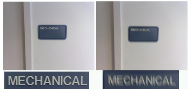
Figure 1. Motion blur example. Top: the same sign is shown in a clear image on the left and in a motion blurred image on the right. Bottom shows text zoomed in from above images: on left, text is clear enough for correct OCR result; on right, blurring causes incorrect OCR result (“MIOHANICAL”).
