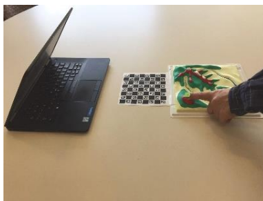
Figure 2: CamIO system shows laptop, object (relief map), fiducial marker board and user pointing to a hotspot.
