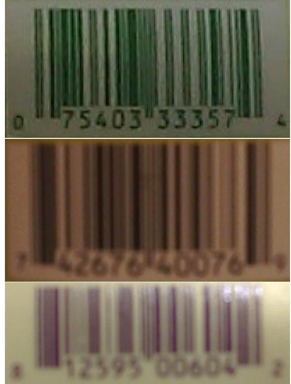
Figure 5. Examples of hard images from our dataset. Top: read correctly only by our algorithm (with modulus less than 2 pixels); middle and bottom: read correctly by no algorithm.
