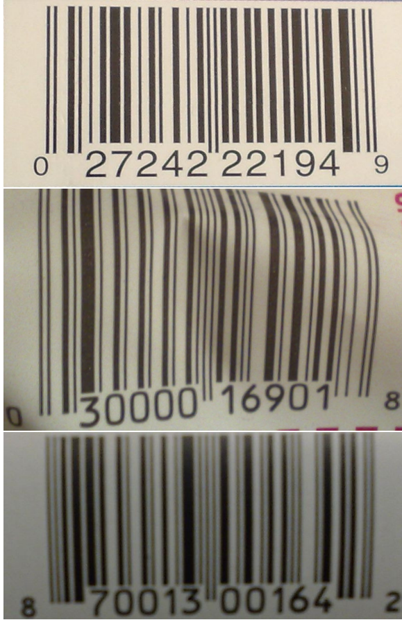
Figure 4. Examples of clean images from our dataset. Top: read correctly by our algorithm and both commercial readers; middle: read correctly by our algorithm and Barcode Decoding Software; bottom: read correctly only by our algorithm.
