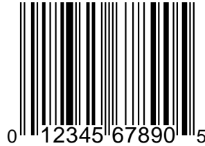
Figure 3: UPC-A 012345-678905. The digits are organized as Ss_1s_2s_3s_4s_5s_6Ms_7s_8s_9s_{10}s_{11}s_{12}E where S and E are the start and end characters, represented by the 3-bit pattern 101, and M is the middle 5-bit guard bar 01010.
