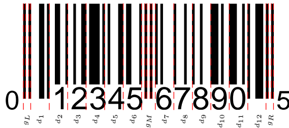
Figure 4: Fixed edges of UPC-A barcode shown as dashed red lines. Labels on bottom denote the guard regions and the 12 digit regions between the fixed edges.
