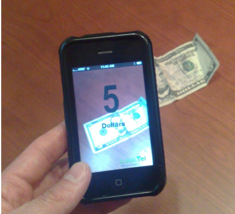
Figure 10.5. LookTel Money Reader, a currency reader app for the iPhone. System detects and reads aloud the denomination of the bill (in this case, $5) in real time.
