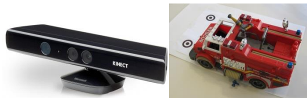
Figure 1. (a) RGB-D camera (Kinect) used in current CamIO prototype. (b) Toy truck model used in experiment.
