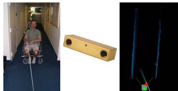
Figure 1. (a) Wheelchair system. (b) Close-up of stereo camera, which is mounted above wheelchair rider's head. (c) Elevation map estimated by system shows corridor walls (long blue lines) and the cane (long white line near bottom).
