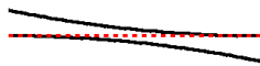
Fig. 1. Two slightly curved lines (black), representing edges of crosswalk stripes (with exaggerated curvature). The straight red dashed line is tangent to both lines, which means that the Hough transform cannot resolve the two black lines separately.
