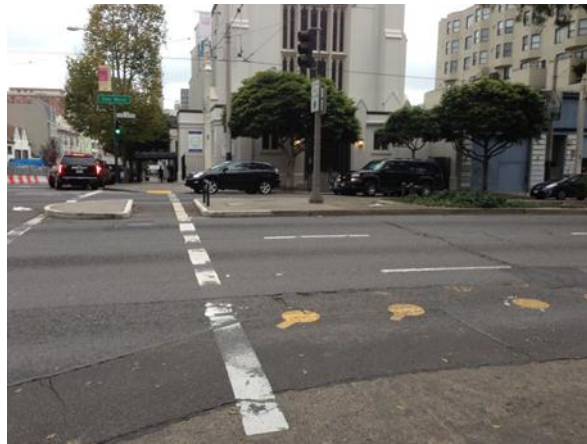
Figure 1. Some important intersection features are difficult to detect reliably using computer vision at typical viewing distances. One such example is the raised median (shown in picture), which is an elevated portion of a street that often serves as a place for pedestrians to pause while traversing a crosswalk. We propose that it is more practical to determine the presence of the median and a variety of other intersection features using data from a GIS.
