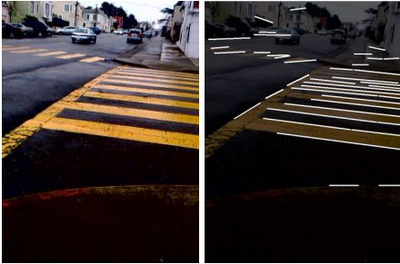
Figure 2. Left, picture of zebra crosswalk. Right, straight-line segment features extracted from image (superimposed in white).
