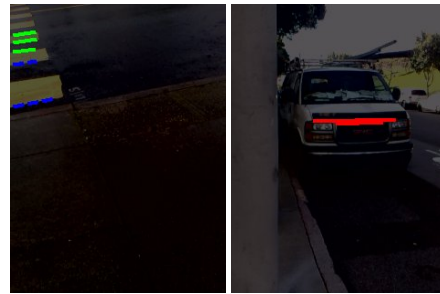
Figure 6. Left, the only image in the test set that was misclassified as not containing a crosswalk. Right, the only image in the test set without a crosswalk that generated any false positive segments (but too few for the entire image to be misclassified), shown in red.
