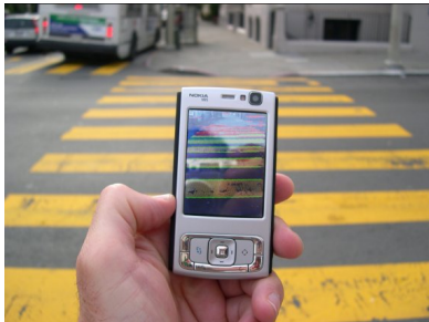
Figure 7. Photograph of Nokia N95 cell phone running crosswalk detection algorithm. The green and red lines superimposed on the crosswalk stripe edges in the cell phone display denote segments classified as figure and ground, respectively.
