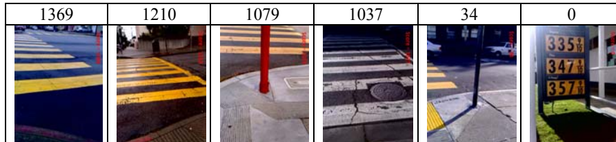
Fig. 3. Images ranked according to the score assigned by the crosswalk detection algorithm; scores (printed above each image) decrease from left to right. The first four images are above threshold (and are thus classified as containing crosswalks), while the last two are below threshold (and are thus classified as not containing crosswalks).
