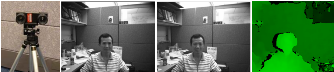
Figure 1 (a) Stereo video camera. (b) Left image. (c) Right image. (d) Disparity map d(x,y) produced by stereo algorithm: brighter green means higher disparity and thus closer to camera; black pixels indicate no estimate at that location. The disparity map clearly shows that the person in the images is closer to the camera than the walls behind him.
