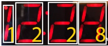
Figure 1. Sample LED display contains a string of digits, each of which is a standard seven-segment digit. For each digit, our algorithm estimates its bounding box (shown in white) and then reads it (results in yellow).
