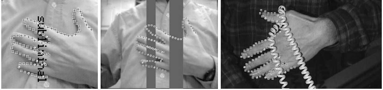
Figure 14: Examples of occlusions. In these figures, the occlusion state at each point is designated as follows: a '+' means state 0 (i.e. unoccluded), a ' \lambda ' means state 1/2 (triple point), and a circle means state 1 (occluded).
