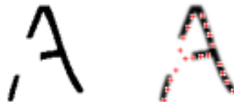
Fig. 5. Robustness of template to partial occlusion. (a) Image contains an A missing its middle left corner and portions of adjoining segments. (b) DQ is able to recover the missing points (red and white crosses), enabling a successful detection.
