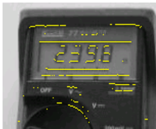
Figure 3: Horizontal edge pair pixels: when two edge pixels of opposite polarities are next to each other, an edge pair pixel is constructed, located between them.
