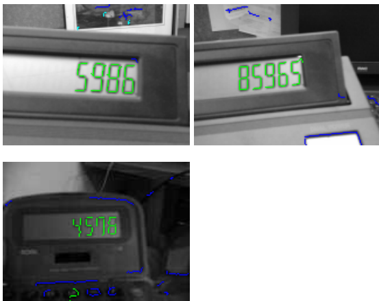
Figure 7: Experimental results for LCD displays. Stroke clusters assigned to "figure" are shown in green and "ground" in blue. False positive in bottom of last image is rejected by the algorithm for reading individual digits.
