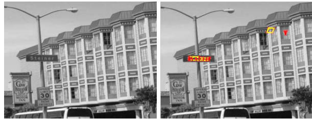
Figure 10. Most common false positives: periodic structures such as rows of windows resemble text at a local scale.
