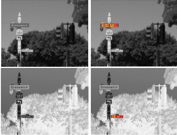
Figure 7. Polarity selectivity. Top: algorithm finds light text on dark background. Bottom: by inverting the contrast of input image, text of opposite polarity is detected.
