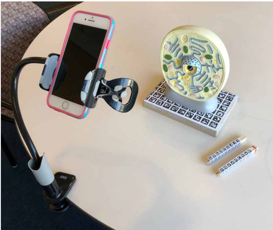
Fig. 1. CamIO system overview. A 3D biological plant cell model is mounted on the CamIO board barcode pattern. The reading and writing styluses (the writing stylus has a red rubber band on its end) are next to it. The CamIO app is running on the iPhone 8, held by a gooseneck cell phone holder clamped to the table, with its main camera aimed towards the cell model.
