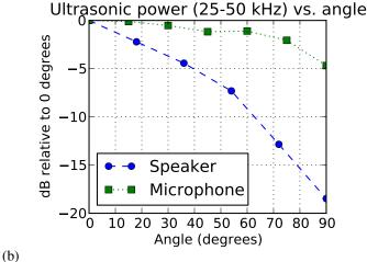
Fig. 3. Measurement of transfer functions for ultrasonic microphones and ultrasonic speaker as a function of angle. (a) Angular transfer function measurement setup. (b) Angular transfer function data. For the microphone, the sensitivity relative to the sensitivity at zero degrees is plotted; for the speaker, the emission power relative to the emission power at zero degrees is plotted.
