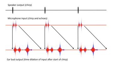
Fig. 2. Schematic of waveforms at several processing stages, from ultrasonic speaker output to stretched pulse-echo signal headphone output presented to user. Red traces correspond to the left ear signal, and blue traces to right ear signal. Note that the relative temporal scales are chosen for ease of visualization, and do not correspond to the temporal scaling used experimentally.
