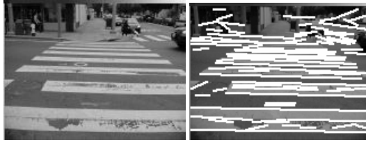
Fig. 2. Left, typical intersection image photographed by camera phone. Right, straight-line segments extracted from image shown in white.
