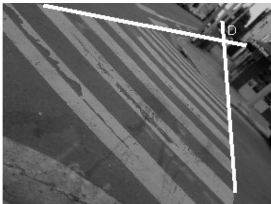
Fig. 6. Severely tilted crosswalk image could be misleading. Vanishing point, labeled D , is on the right side of the image even though the camera is aligned to the crosswalk.
