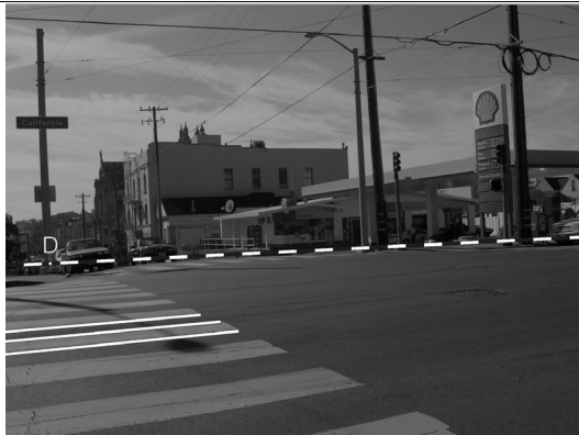
Fig. 5. Determining the horizon and vanishing point when only one of the two borders of the crosswalk is visible. The three solid white lines are the crosswalk edges used to estimate the horizon (dashed white line) and the vanishing point (white dot on horizon line, labeled D ).
