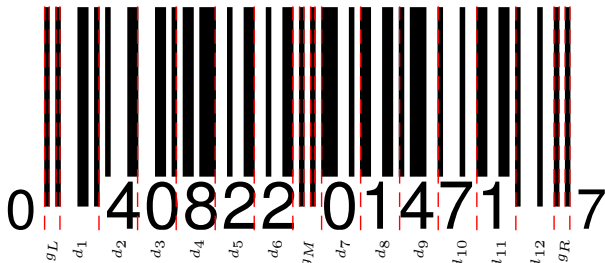
Figure 2. UPC-A barcode, encoding 12 digits. The code axis runs left to right in this image and the bar axis runs vertically upwards. Note that the the bar patterns representing any specific digit have opposite polarity on the left and right sides of the barcode.
