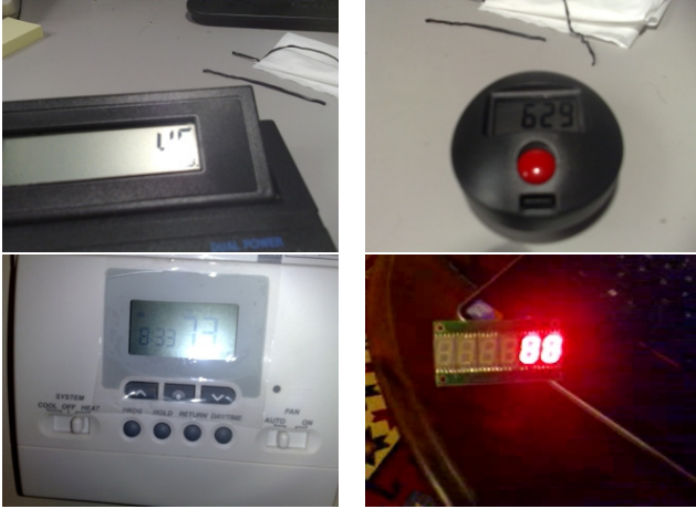
Figure 1. LCD's can suffer from glare and low contrast, whereas LED's can saturate images.
