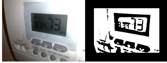
Figure 2. Result of binarization on LED screen
