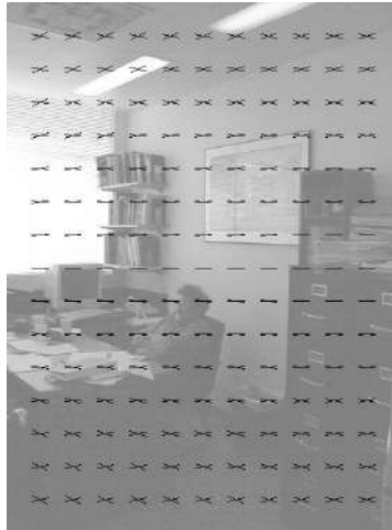
Figure 4: Another indoor scene. Standard conventions for display of \vec{i}, \vec{j} directions. Observe that the \vec{i}, \vec{j} directions align with the appropriate walls despite the poor quality of the image (i.e. under-exposed). (Indoor 15).
