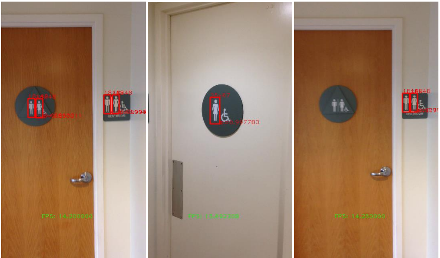
Figure 2. Sample Restroom sign detections. Note that the current Restroom detector captures both Men's and Women's icons; in the future we will create an additional classifier to distinguish between the two genders. The third image illustrates two false negatives, i.e., two Restroom icons that are not detected.
