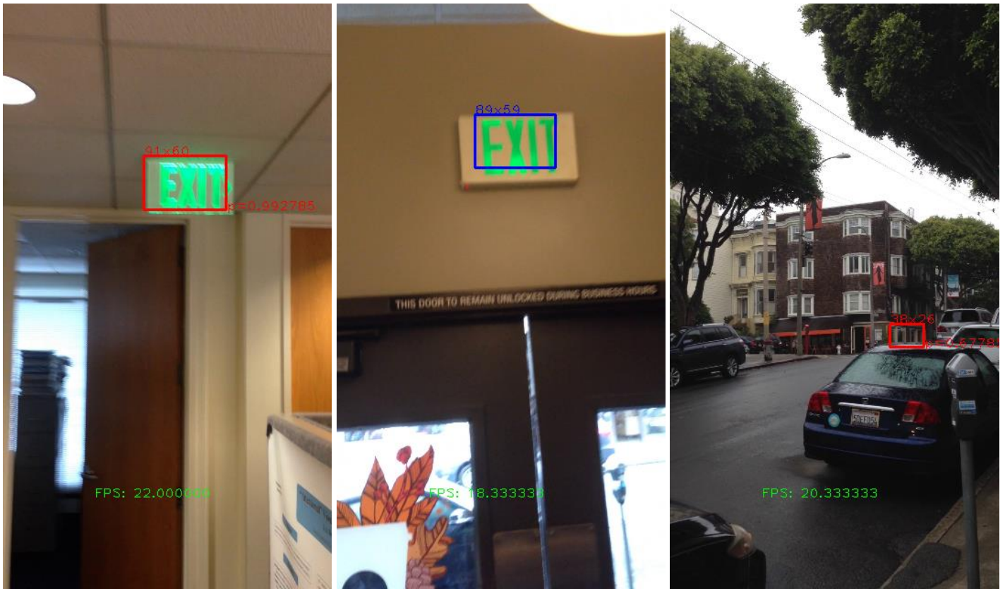
Figure 1. Sample Exit sign detections. From left to right: (a) Successful detection. (b) Blue rectangle shows a false negative (missed detection), indicating a candidate detected by the first (Adaboost) classifier stage that is incorrectly rejected by the second (SVM) classifier stage. (c) False positive (spurious) detection shows a region with texture from building façade.
