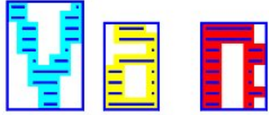
Figure 1. Blobs as a collection of horizontal line segments
